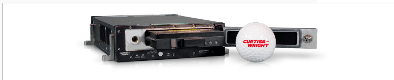
Figure 2 - 1 GbE NAS Example (DTS1)
